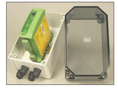
**BOX 2/4 IP66** control unit together with the Safety Light Curtains TYPE 2 (model OPT3 SMC PXXX) upgrades the category to TYPE 4.
