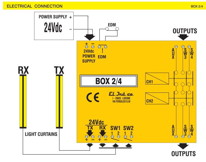
**N.B.** The unit "BOX 2/4" is provide with the EDM function temporarily disabled (jumper on terminal EDM).
